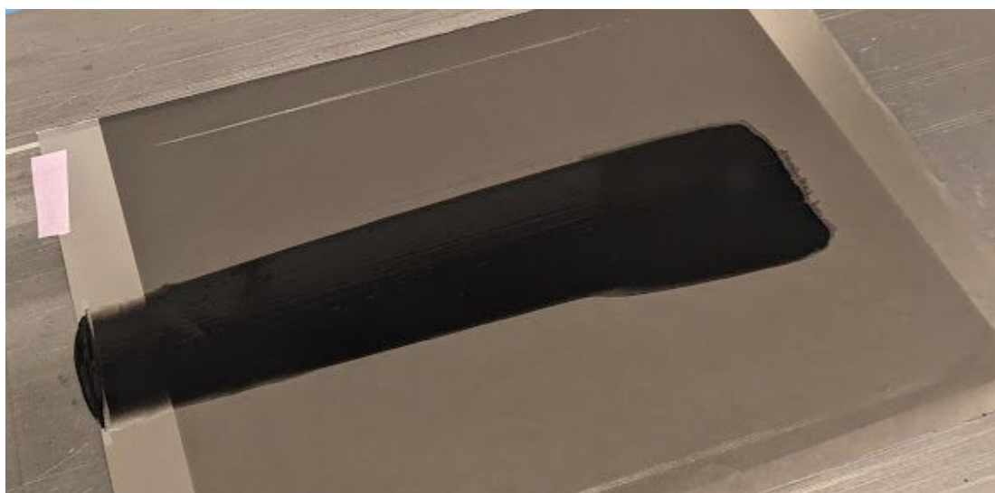
Figure 5: Casting of slurry for coin cell cathode
